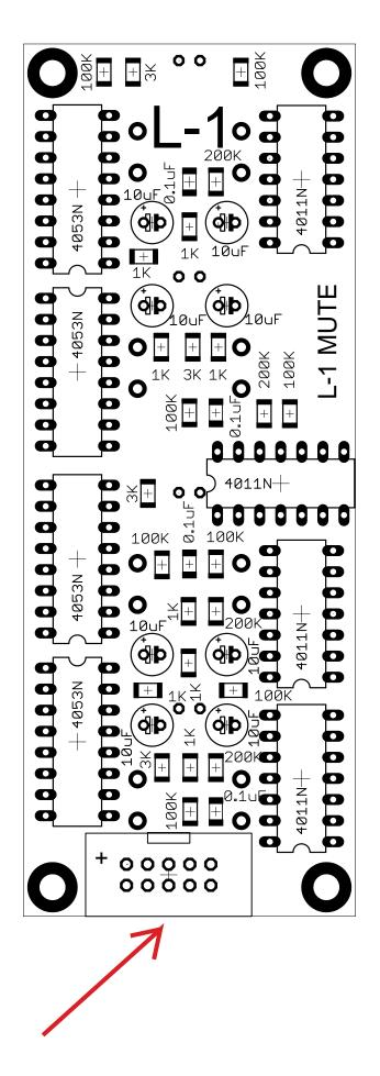
Connect to connector on the right side of the VC Stereo Mixer. Don't connect to a power line.
