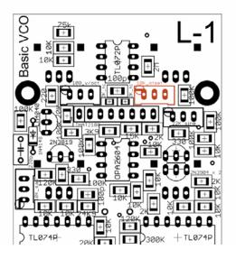
This trimpot just sets offset voltage. Turn COARSE pot to min, FINE pot to max. Trim to desired note, CO for example.
