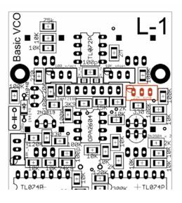
Adjustment of symmetry of the sine wave.
